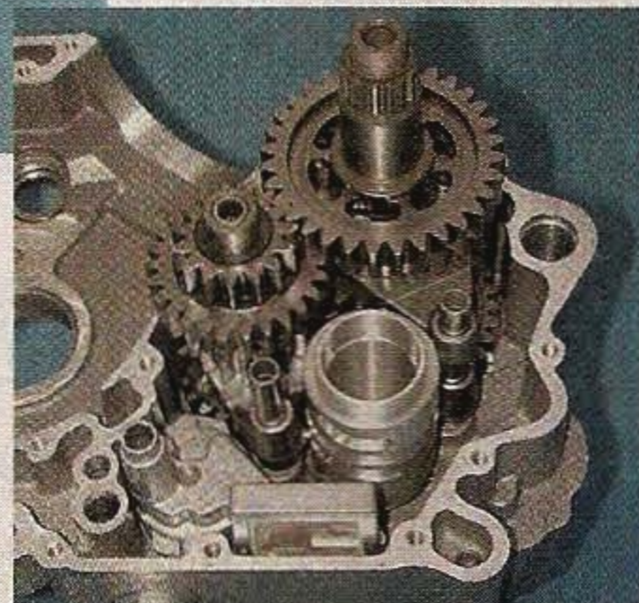
Above: The vertically split crankcase displays its center-mount electric-starter assembly. Above, right: Cylinder heads are much smaller than those of KTM's competitors. Right: Six-speed tranny will be standard on both bikes. Far right: LC8 crankshaft is light and connects to nearly skirtless pistons.
